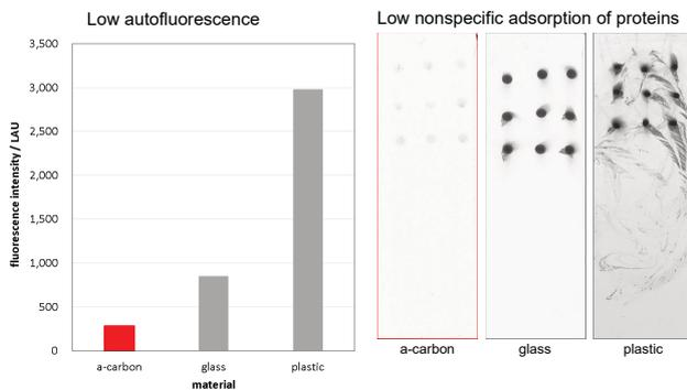
**Figure 1:** Autofluorescence of plate materials. Measurement instrument : FLA8000 ex. 532nm, em. 570nm
